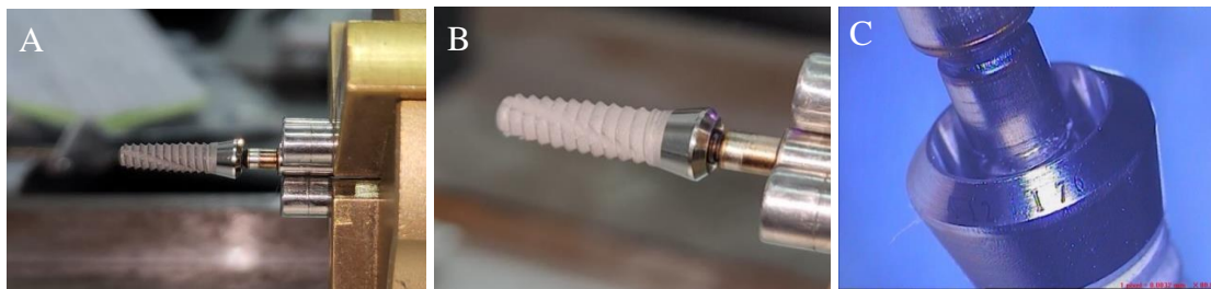
Fig. 14a. 14b. Implant Morse taper with external polish, pre-engraved and while engraved. Fig. 14c. Morse taper implant polished exterior surface, post-engraved. Source: Laboratorio Romi, S.A. Quilmes, Argentina.
