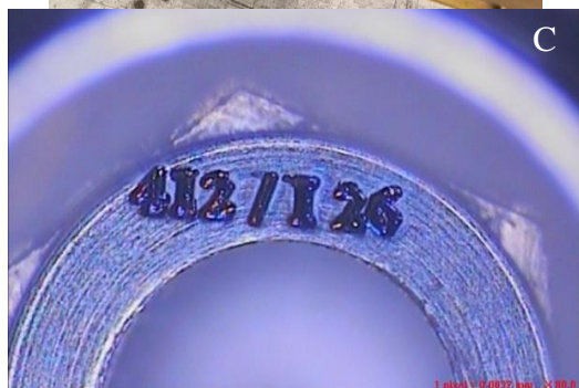
Fig. 11a. 11b. Inner surface of Internal hexagon implant, pre-engraved and during engraving. Fig. 11c. Internal hexagon implant on the inside surface, post engraved. Source: Laboratorio Romi S.A., Quilmes, Argentina.
