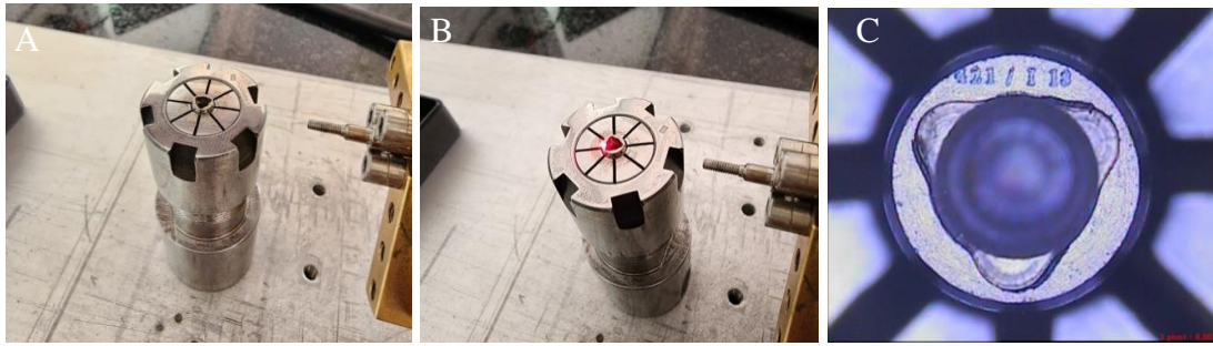
Fig. 13a. 13b. trichannel implant inner surface, pre-engraved and while engraving. Fig. 13c. Trichannel implant inner surface, post-engraving. Source: Laboratorio Romi S.A., Quilmes, Argentina.
